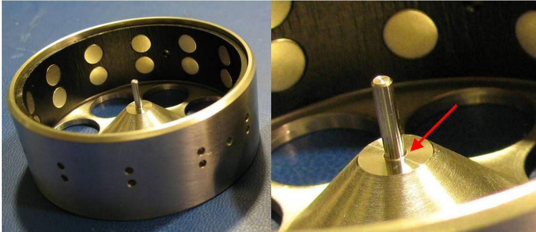
*Figure 3: One-Piece Wheel, Showing Stress Concentration at Shaft Root*
