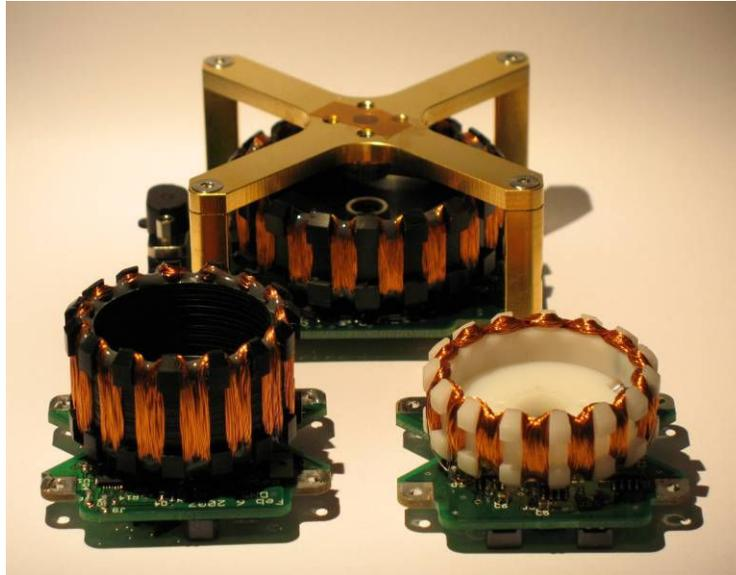
Figure 2: Electronics units from RW-0.03 (left), RW-0.01 (right) and RW-0.06 (rear)
