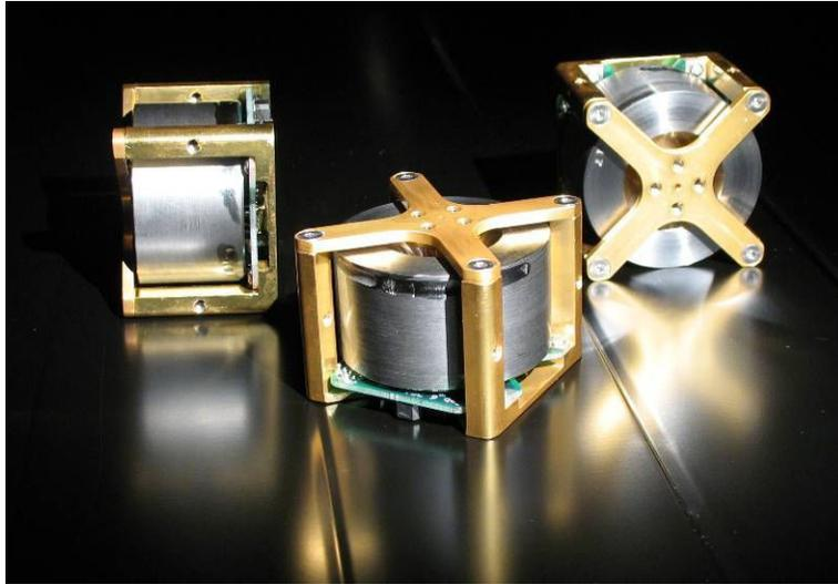
*Figure 1 Three GNB Reaction Wheels*
