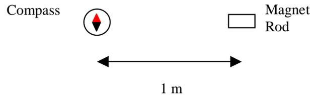
Figure 7: Dipole Measurement Method
