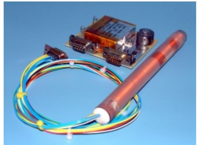
**Figure 2: Magnet Rod and Drive Electronics**
