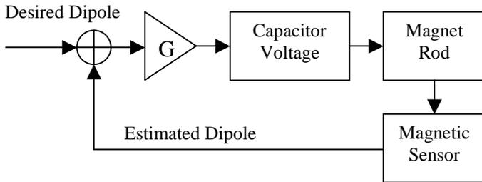
**Figure 4: Closed-Loop Control**
