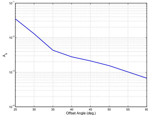
Figure 7: Predicted baffle attenuation (adapted from<sup>15</sup>).
