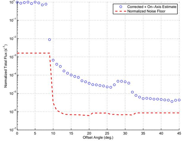
Figure 3: Off-axis performance attenuation measurements.
