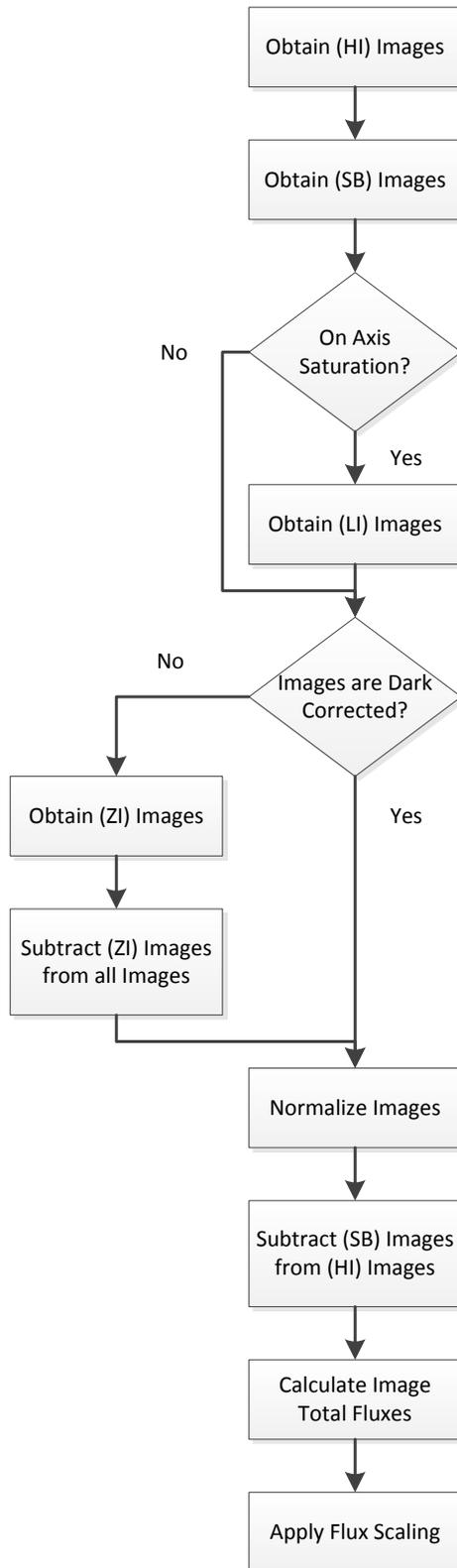
Figure 1: Overview of the Stray Light Test.
